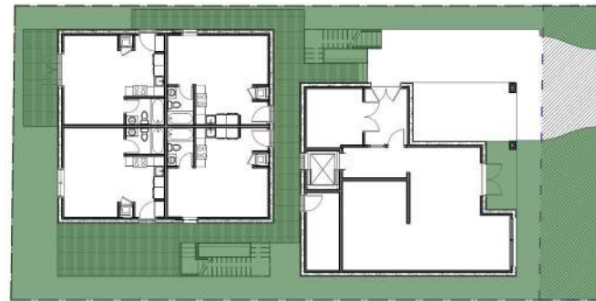
6 Open Site Space Scale: 1:200 Open Area 256.7 m 2 Site Area 586.27 m 2 Site Coverage 43,7%
