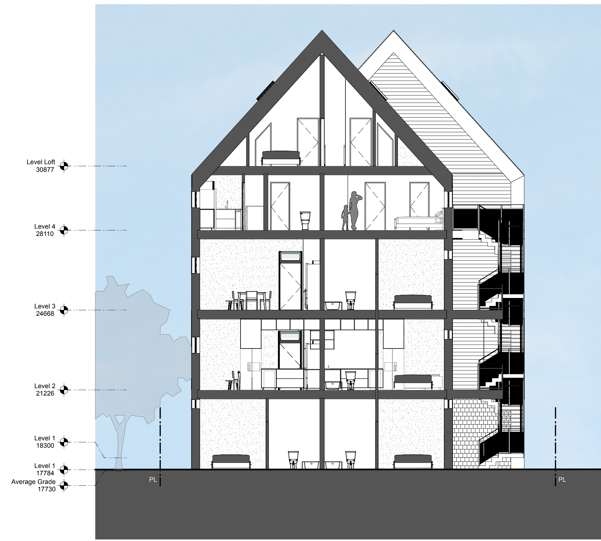
3 Building Cross Section Scale: 1:100
